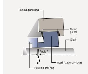
With Flowserve's flexibly mounted insert, the gland ring can be cocked and the insert remains square with the axis of the shaft.
