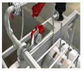
The oscillating spray bar backwash system and the integrated level tank are some of the specific design details that make the SuperDisc<sup>™</sup> a reliable and low-maintenance filtration unit with more operational control.
