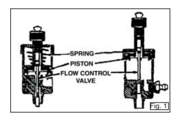
If Gun-Fil® discharges lubricant too rapidly when almost empty, valve should be backed-off or unscrewed 2 or 3 turns to reduce delivery rate slightly. The lubricant feed is controlled by adjusting the travel of the flow control valve. Backing-off the valve restricts the flow for a longer time, preventing excess delivery. When valves are properly adjusted, Gun-Fil® lubricators seldom leak or overlubricate a bearing.
