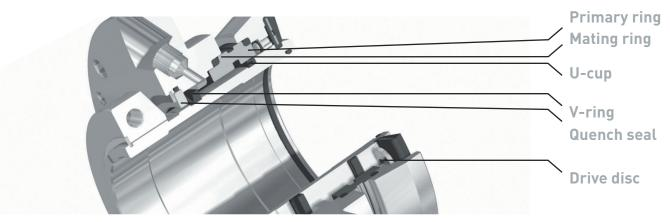
In these premium-material designs, the seal face provides maximum stability and minimum heat generation under adverse conditions, optimizing performance with maximum seal face life and lubrication, outperforming conventional materials.
